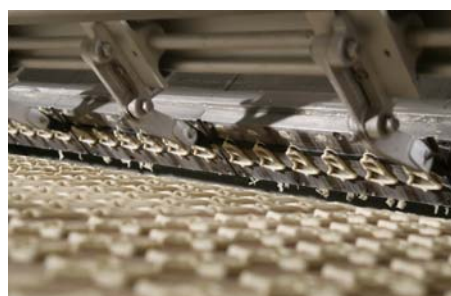
The LP Extruder is a flexible platform for production or new snack development. Shapes may be tested on single die plates and modified to exact specifications before a complete set is ordered.
