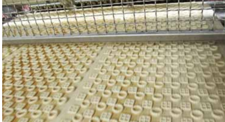
▲ On the pretzel line, a unique double-row die cutter running 265 cuts per minute produces two differently shaped dough pieces simultaneously.
